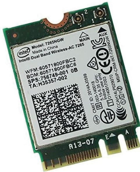
Intel 7265NGW Dual Band Wireless-AC 7265 802.11ac, 2x2 WiFi + Bluetooth 4.0 Card
